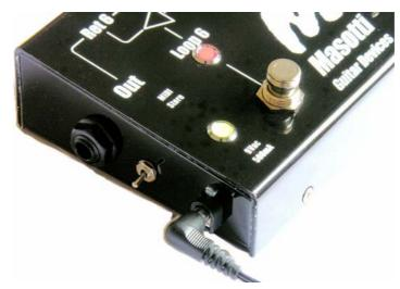
On the left side we can find output jack, programming switch and power supply plug.
